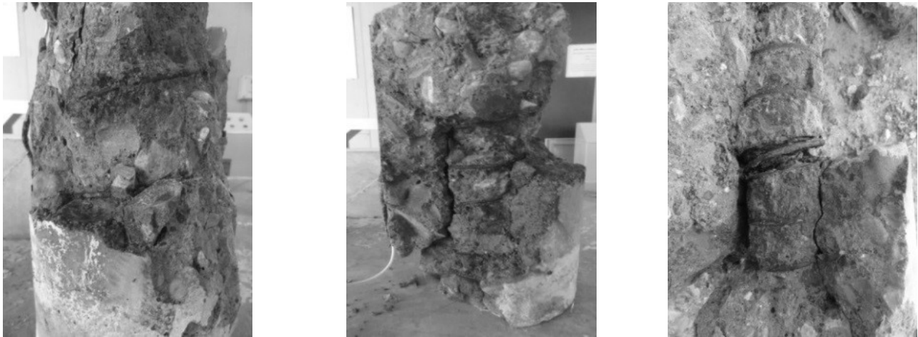
Figure 3. The fracture mechanism of the corroded reinforced cylindrical specimens [25]
